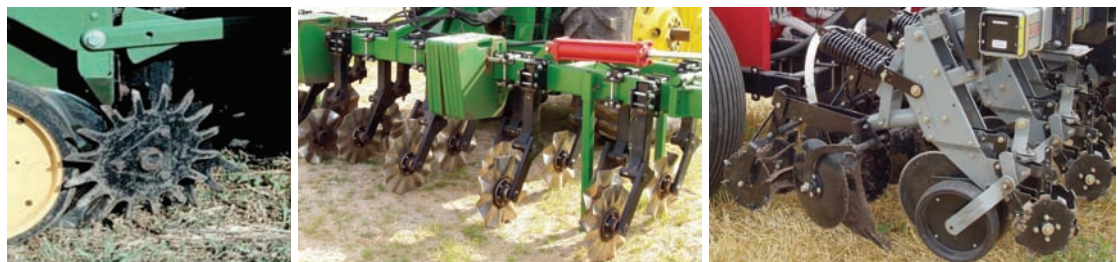
Figure 1. Examples of strip-tillage tool categories (left to right): row-clearing coulters, shallow strip-tillage tool, moderate strip-tillage tool
