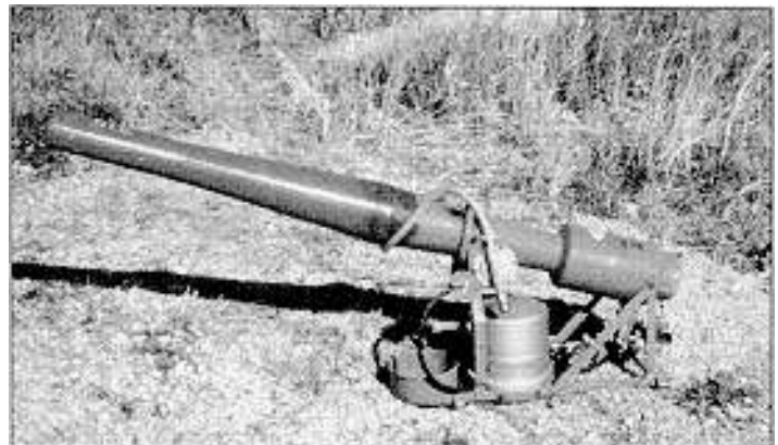
Gas-operated exploders or "cannons" are commonly used tools for abatement of Canada geese damage.
