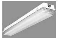
Generally, T-12HO fixtures are used in cold locations (<50°F) which is unnecessary if the correct T-8 ballast has been selected since the T-8 ballasts are designed to work down to 0°F with a few exceptions (check package labeling).
